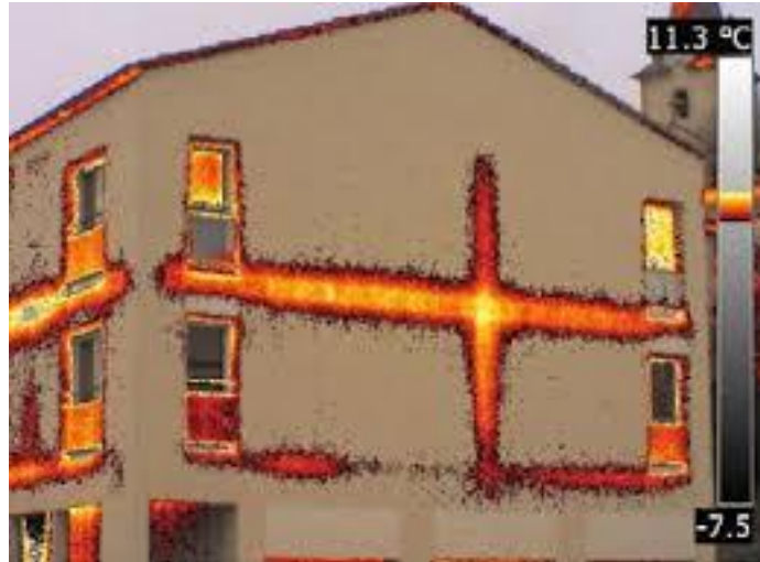
Figure 12 Example of thermal bridges measured by a thermal camera [2]
